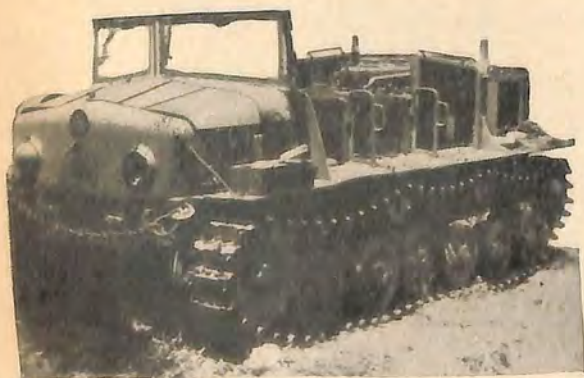
Figure 320. Model 98 (1938) 6 ton prime mover.
